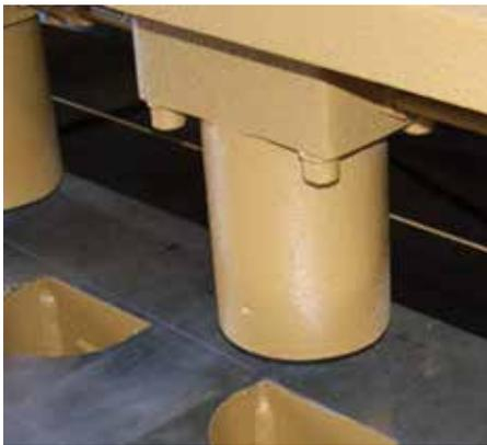
Extremely heavy-duty hold downs. Fewer hold downs = less maintenance. Hold down pressure is adjustable for your sensitive material.
