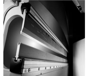
**Conventional Tooling**—Adjustable, conventional, four way, single V plus all other die requirements available with model AB press brakes
